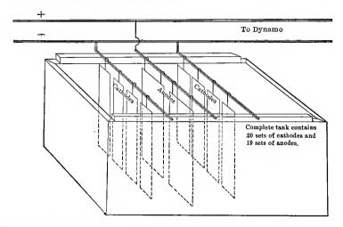
FIG. 8. Refining tank for copper, which is deposited by the current from a copper sulphate solution.
